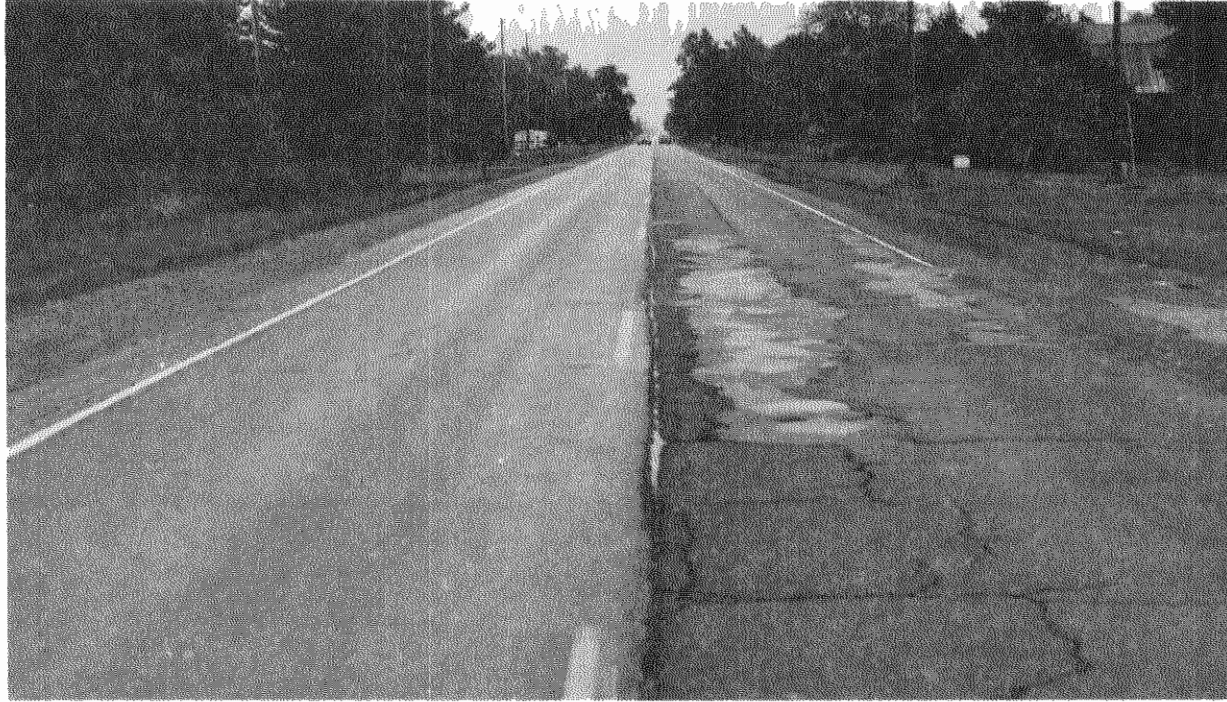
Control section 7 in left lane. Ground rubber mix, 1-1/2 percent, in right lane, section 15.
