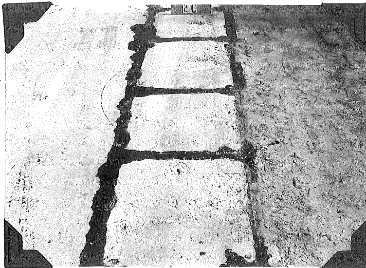
Figure 4B. Calcium chloride panel of test area No. 2 after 26 cycles. Pavement 4 years old containing cement brand No. 2. Project 18-20,C3. Station 500+50. 11 percent scaled.
