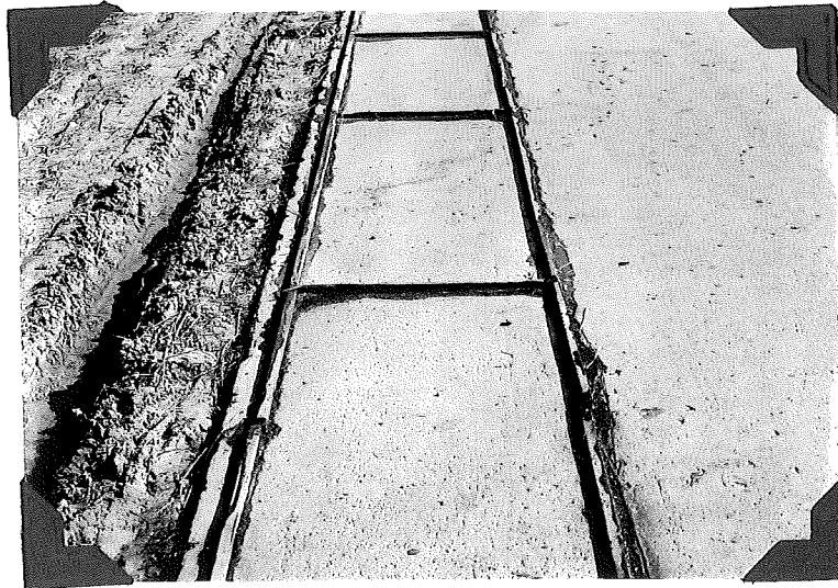
Figure 2D. Rock Salt panel of test area No. 6 after 30 cycles. Concrete 9 years old. No scale.
