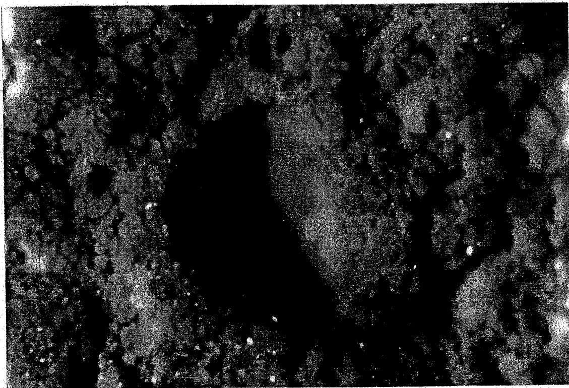
Figure 4. Calcium carbonate incrustations and void linings formed as a precipitate on a partially immersed crushed concrete particle. 20X magnification.
