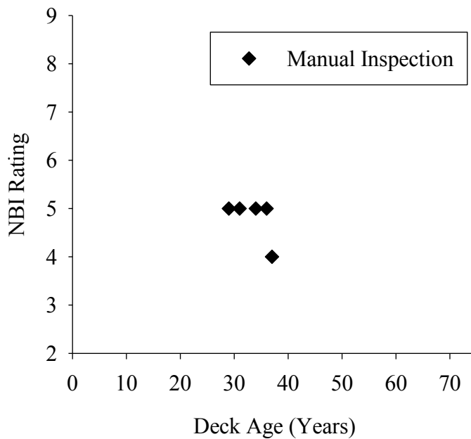
Figure 3-2: Inspection records of bridge 09109035000S130
