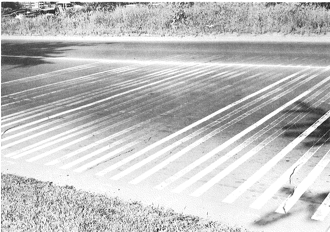
Figure 2. Some white test stripes after one year of exposure. The left stripe of each series of three stripes is reflectorized.
