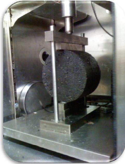
Figure 21 Indirect Tensile Strength Testing Setup
