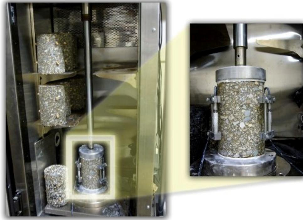
Figure 14 Dynamic Modulus Test Setup
