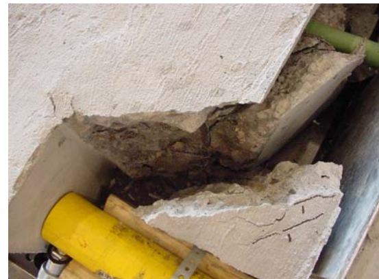
(a) Corner cracks observed in the test specimen
