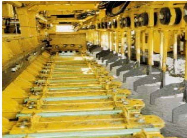
(b) Dowel Bar Magazine in position
