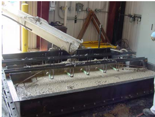
(c) Casting of specimen
