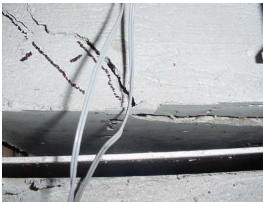
(a) Corner cracks observed in the test specimen
