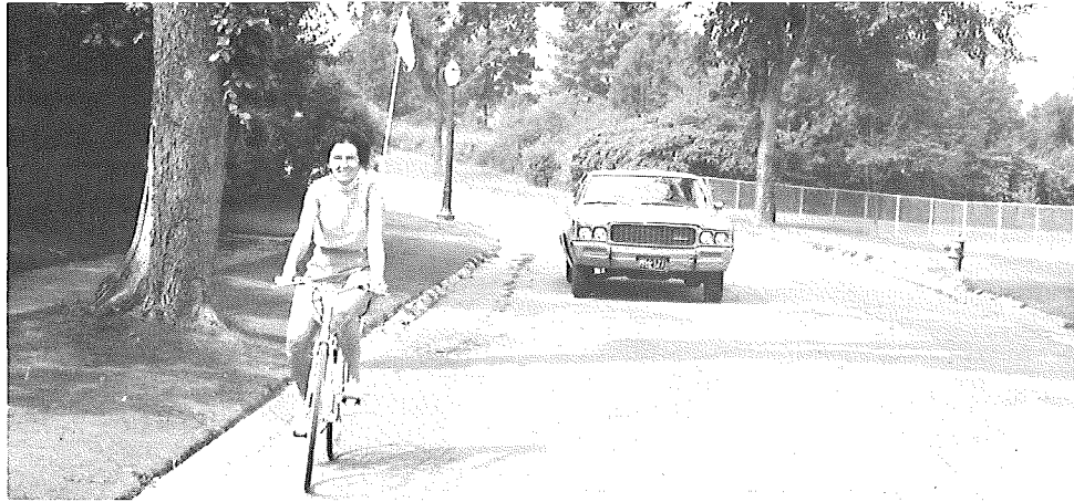
CLASS III – A shared right-of-way, designated as such by "Bike Route" signs placed on verticle posts or stenciled on the pavement. Any bikeway which shares it through traffic right-of-way with moving motor vehicles is considered a Class III bikeway.
