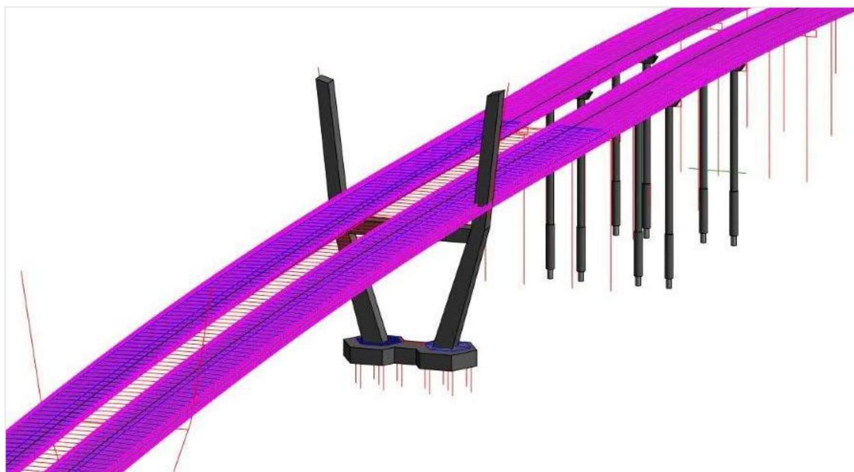
Figure 8: Analysis model used as an underlay for a 3D bridge model.
