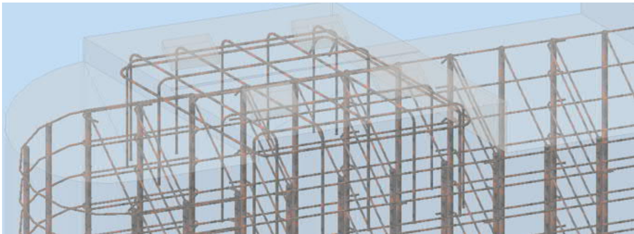
Figure 11: Reinforcement in a parametric model (Brenner, 2015).
