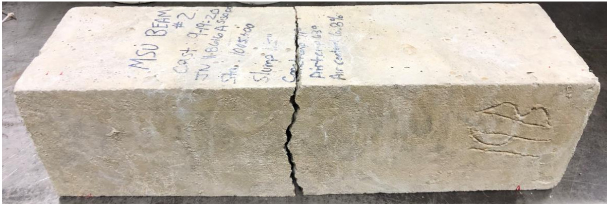
Figure 6-32 Typical beam break – I-196 EB JPCP project
