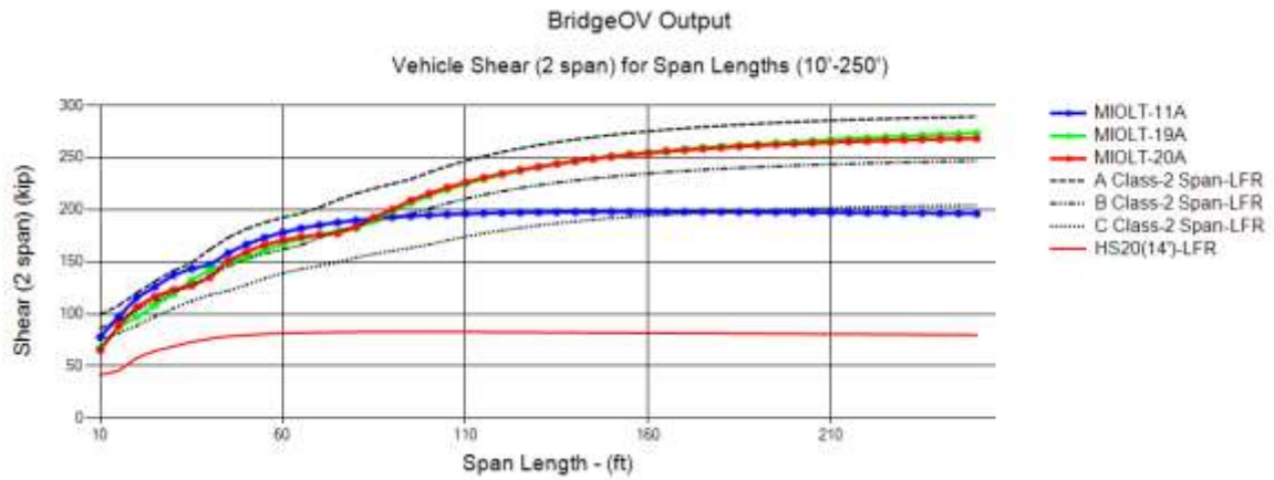
Figure 48. BridgeOV shear-2-span plots – Class A- vehicles 11, 19 and 20
