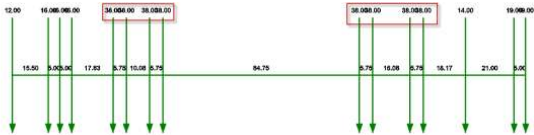
Figure 50. Revised permit vehicle – maximum axle loads changed from 46 kips to 38 kips
