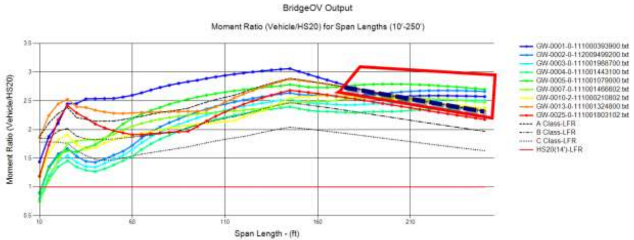
Figure 38. BridgeOV Moment plot for vehicles GW-0001, GW-0002, GW-0003, GW-0004, GW-0005, GW-0007, GW-0010, GW-0013, and GW-0025
