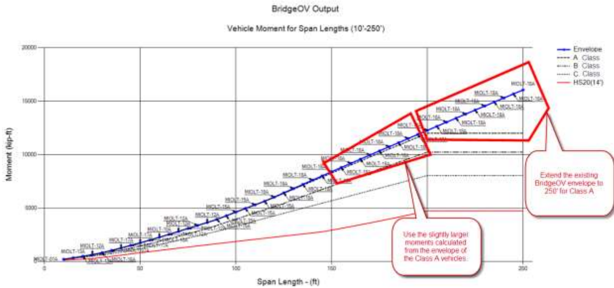
Figure 67. Plot of Michigan Class A moment envelope with the existing BridgeOV Class A,B,C plots (10'-250') NOTE: For this older version of BridgeOV, the Class A,B,C tables ended at 200'
