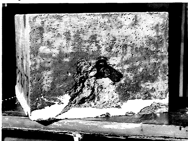
▲ FIGURE 4. TYPICAL FAILURE OF CONCRETE SPECIMEN WITH A ONE INCH DIAMETER DOWEL.
