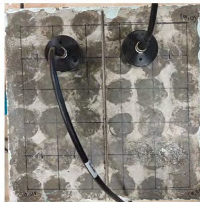
(b) Use of 2-transducer system to measure crack depth
