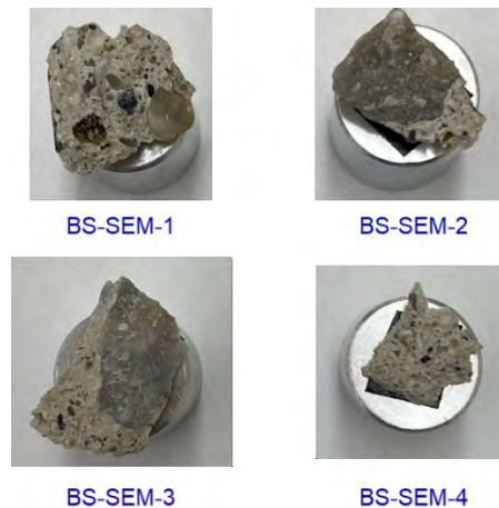
Figure D-12. Specimens for SEM-EDS examination
