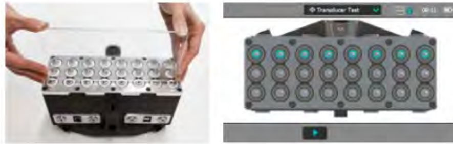
(a) Proceq Pundit 250 array
