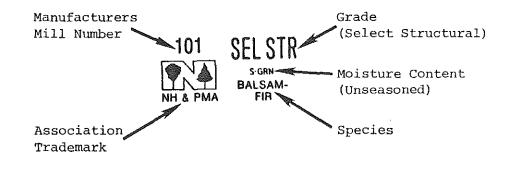
This provides assurance that the material is of a certain quality and that the design stresses can be used with confidence. The use of grade stamped material should correct existing problems in guardrail post procurement. The stamp will also assure that the species is from among the approved list. The use of grade stamps from an approved agency will put the onus of quality assurance on the supplier, rather than on the treating plant or MDOT personnel.
