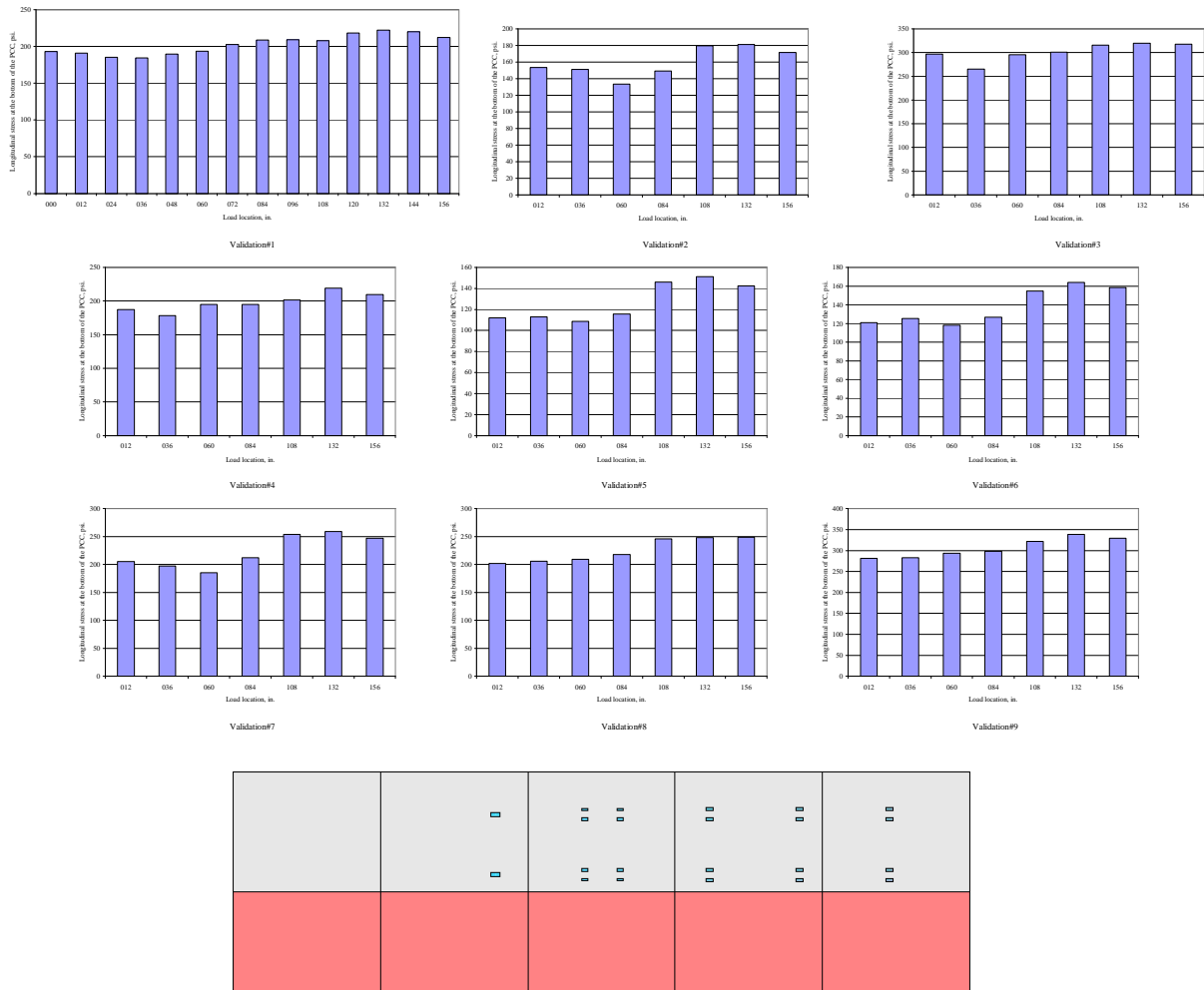
Figure 4-5: Example validation and determination (bottom stresses, MI-9, 177-in. joint spacing)
