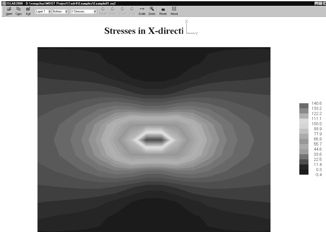
Figure E1-8: Transverse Stress at the Bottom of the PCC Slab
