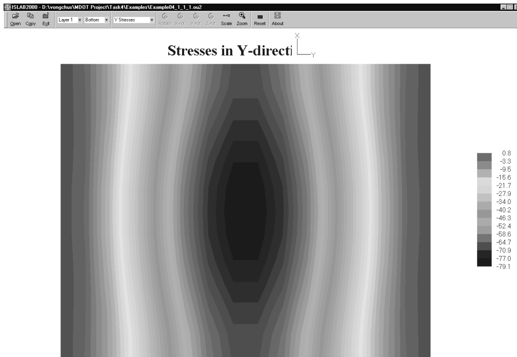
Figure E4-8: Longitudinal Stress at the Bottom of the PCC Slab, \Delta T = -20 °F
