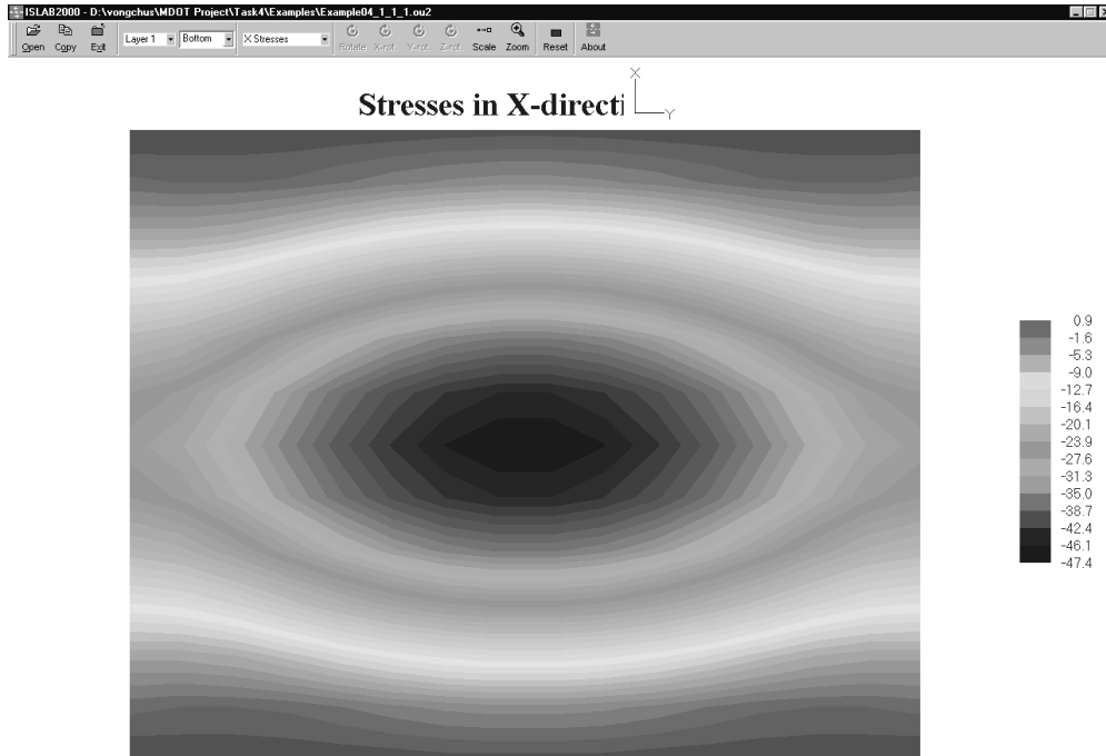
Figure E4-7: Transverse Stress at the Bottom of the PCC Slab, \Delta T = -20 °F
