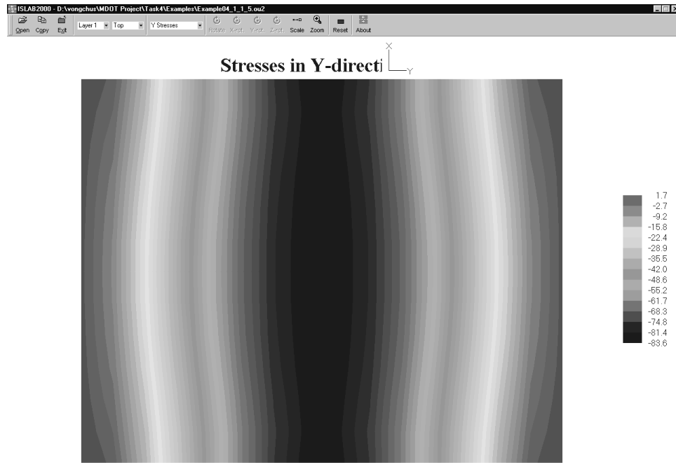
Figure E4-11: Longitudinal stress at the top of the PCC slab, \Delta T = +20 °F
