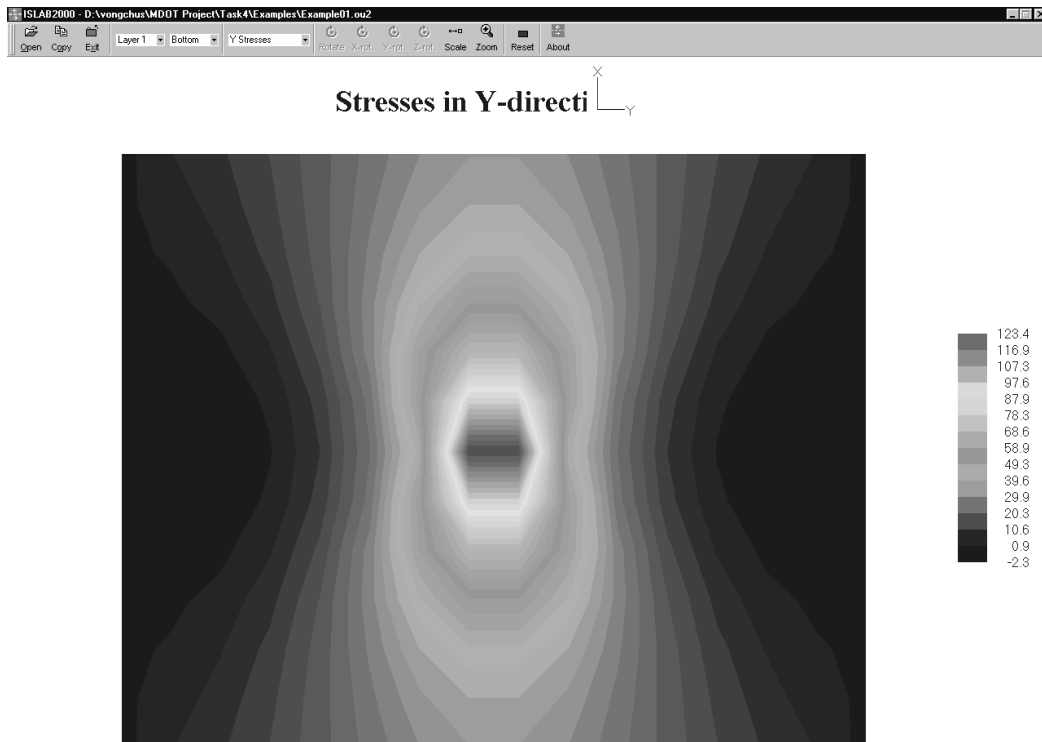
Figure E1-9: Longitudinal Stress at the Bottom of the PCC Slab
