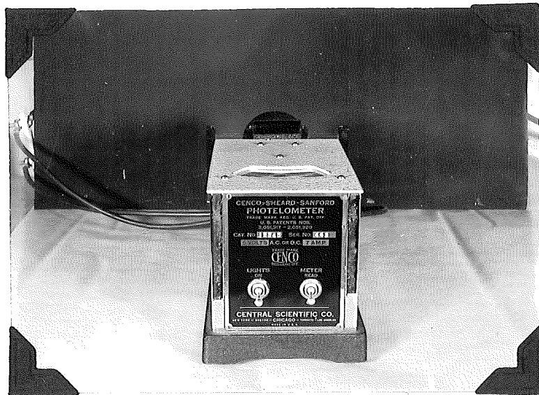
Figure 3. Photoelectric colorimeter suitable for estimating quantities of m-dinitrobenzene. Electric leads are from power supply beneath table.
