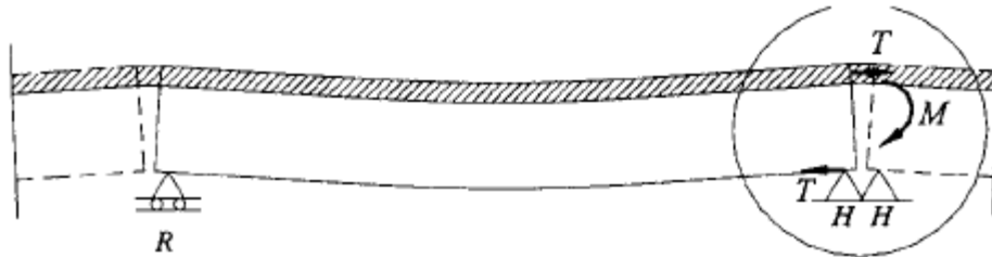
Figure F-3. Effect of RHR type support condition on continuity (Okeil and El-Safty 2005)
