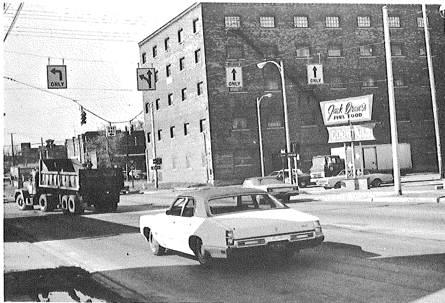
Note truck passing through intersection on "red" while opposing movement is momentarily held back.
