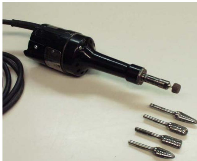
Figure 2-16. Burr grinder and carbide burr tips (Dexter and Ocel 2013)
