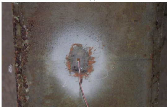
(b) a strain gauge at girder bottom flange
