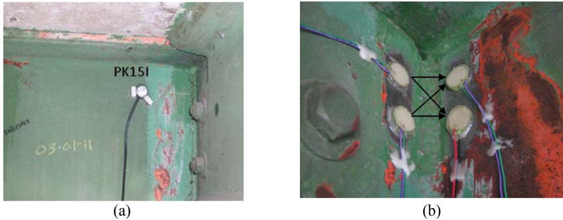
Figure C-2. Sensor locations of (a) AE sensor and (b) USGW sensor array (Zhao et al. 2013)
