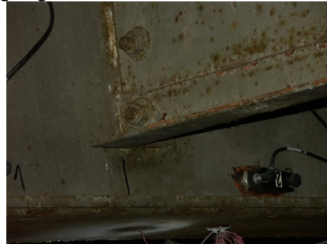
(b) a strain gauge at girder bottom flange
