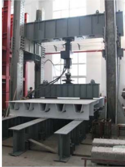
Figure C-13. Experimental set up of the orthotropic steel bridge deck (Yi et al. 2012)
