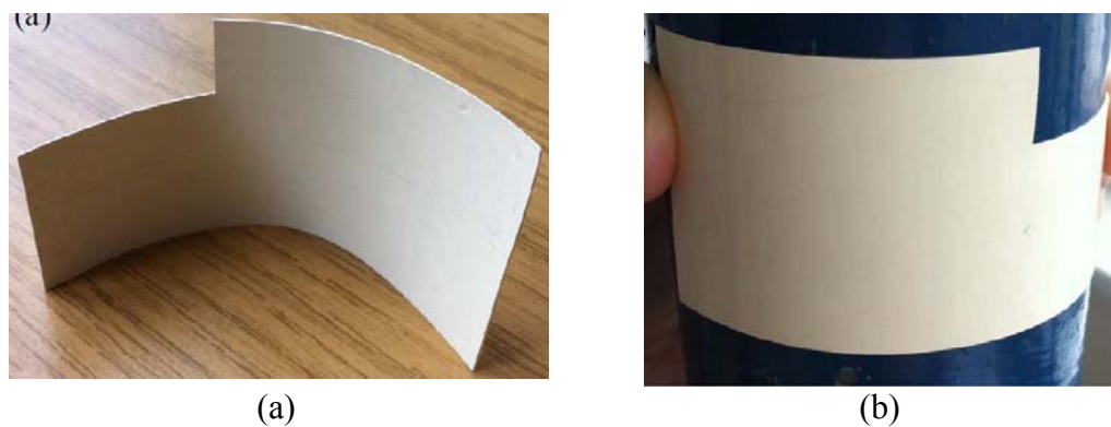
Figure C-5. (a) PZT sensor sample and (b) PZT sensor sample on a curved surface
