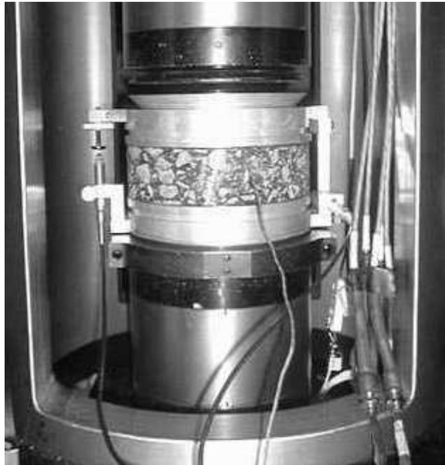
**Figure 2.10 Superpave Shear Test Specimen**
