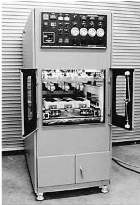
**Figure 2.15 Asphalt Pavement Analyzer**
