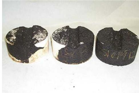
**Figure 6.4 APA Specimens with Plaster of Paris**
