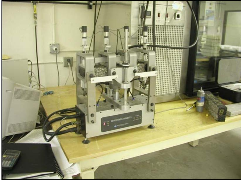
**Figure 6.8: IPC UTM 21© Beam Fatigue Apparatus**
