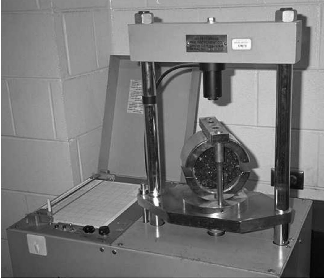
**Figure 2.5 Marshall Stability and Flow Test**
