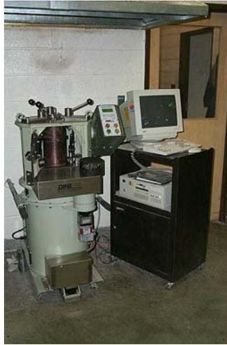
**Figure 6.1 A Pine Superpave Gyratory Compactor**
