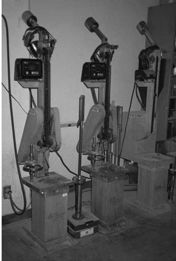
**Figure 2.4 Marshall Mechanical Hammer and Pedestal**
