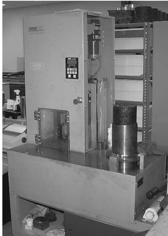
**Figure 2.6 Superpave Gyratory Compactor**
