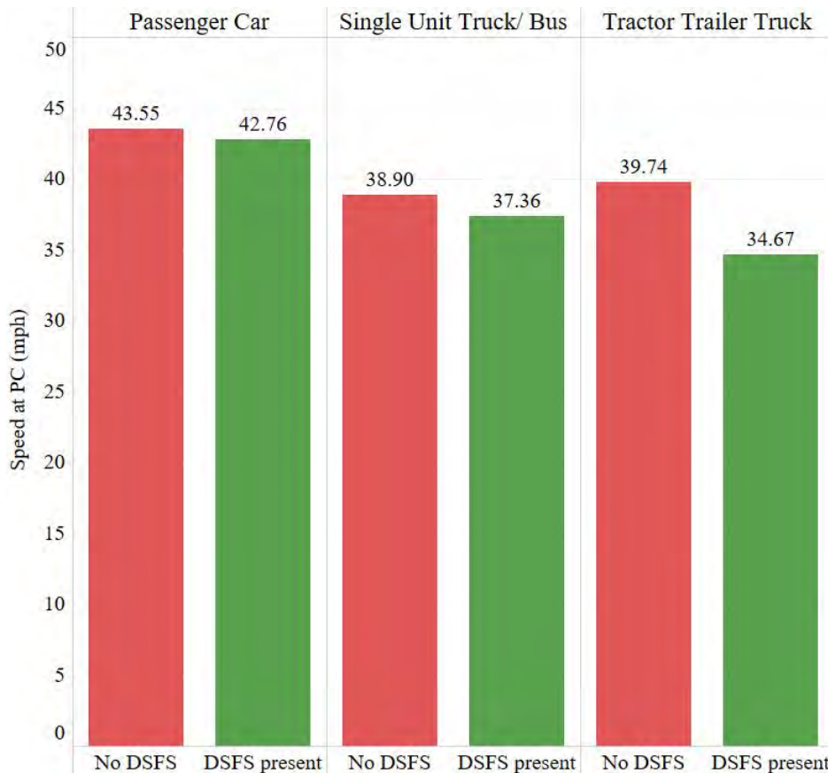
Figure 14. Mean curve entry speeds by DSFS presence and vehicle type
