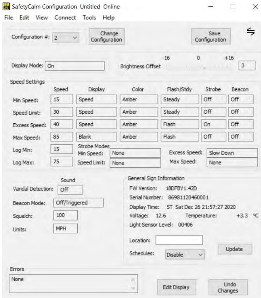
Figure 5. TrafficCalm sign programming using SafetyCalm software
