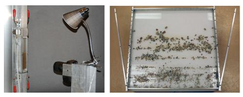
Sedimaging (left) statistically calculates aggregate particle sizes from camera images of samples that have been settled by water. The tilting, backlit Translucent Segregation Table process (right) uses images to calculate the size of each particle on the table.
