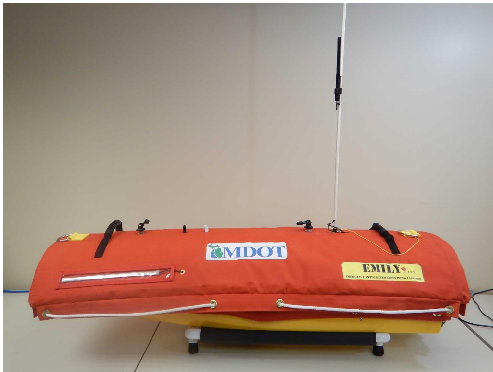
Figure 6: Sonar EMILY with float and antenna installed
