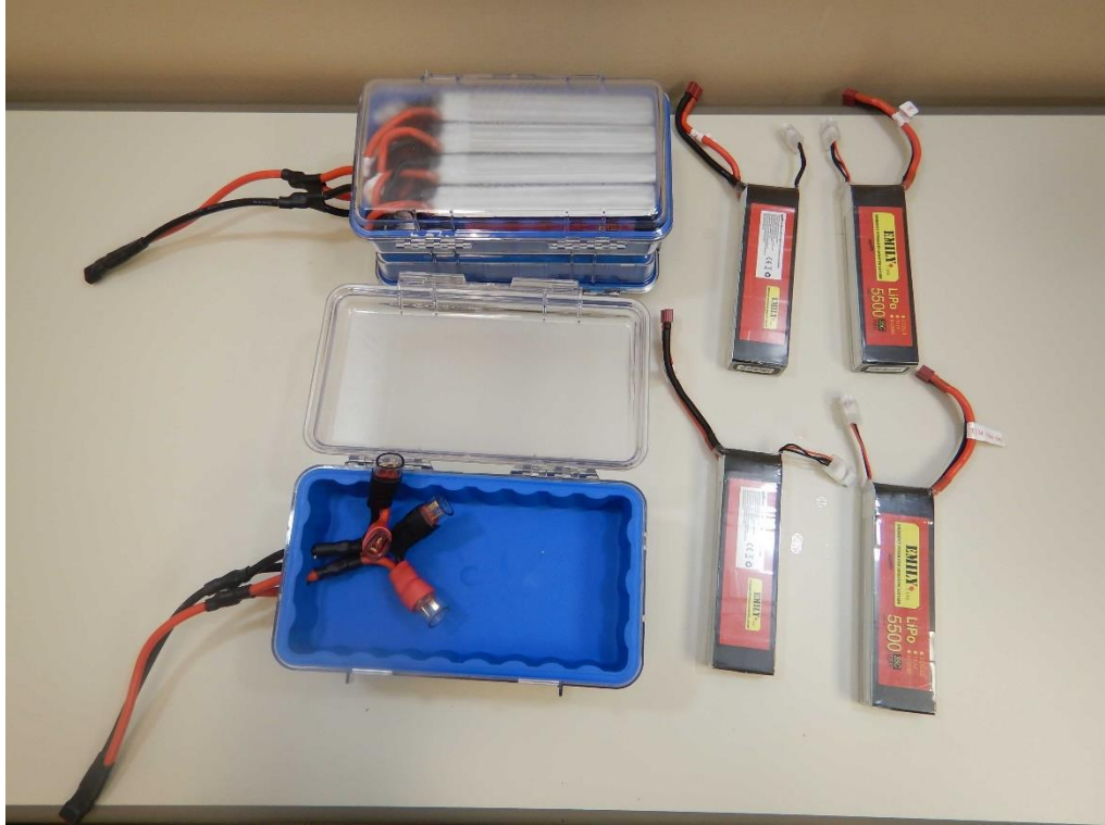
Figure 9: Batteries and Waterproof Case
