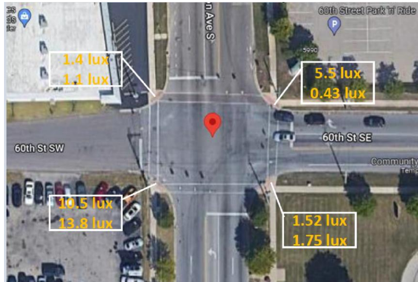
Figure 4-13. Site layout and light readings at the intersection of Division Ave and 60th Street, Grand Rapids
