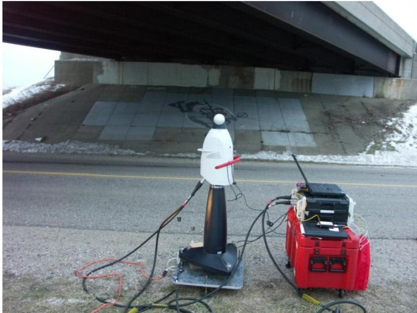
**Figure 3-28. Laser Tracker, server, and computer**
