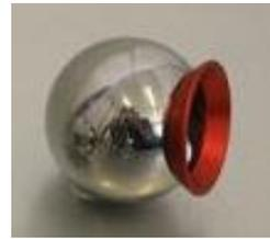
(a) 0.5 in. glass prism reflector      (b) 1.5 in. red-ring reflector (RRR)
