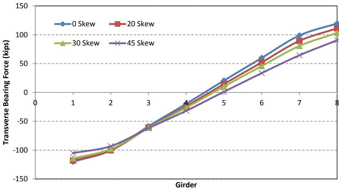
Figure 5-23. Transverse bearing force over abutment under thermal contraction strength load combination
