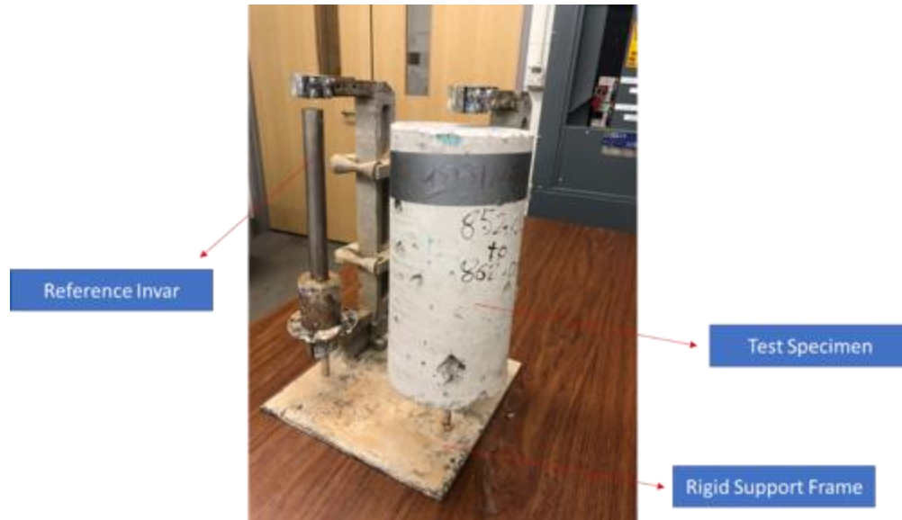
Figure 56 Calibration bar (left) and test specimen (right) seating on the rigid support frame
