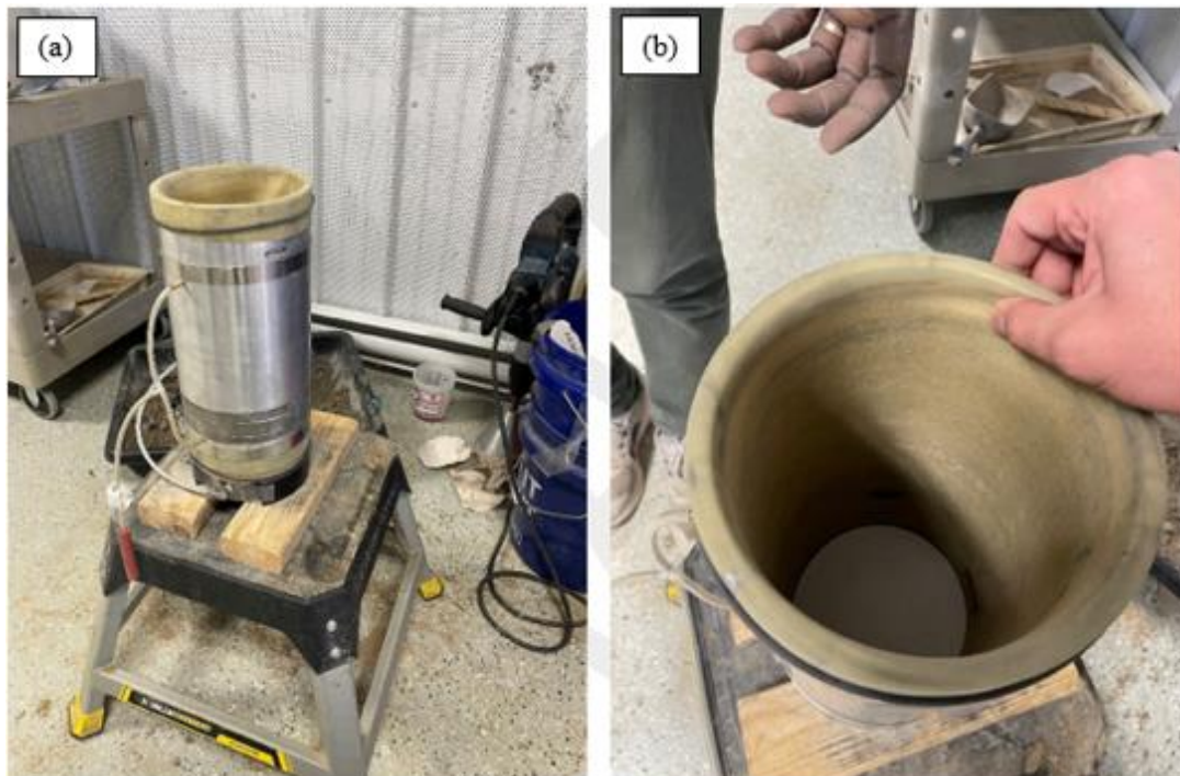
Figure 71 (a) Compaction mold setup and (b) inside of the mold
