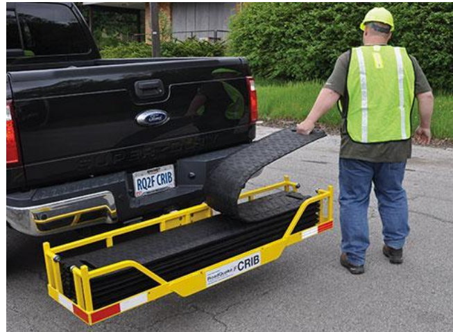
Figure 20. Transport of Portable Temporary Rumble Strips (Photo Credit: Portable Temporary Rumble Strips of Virginia)
