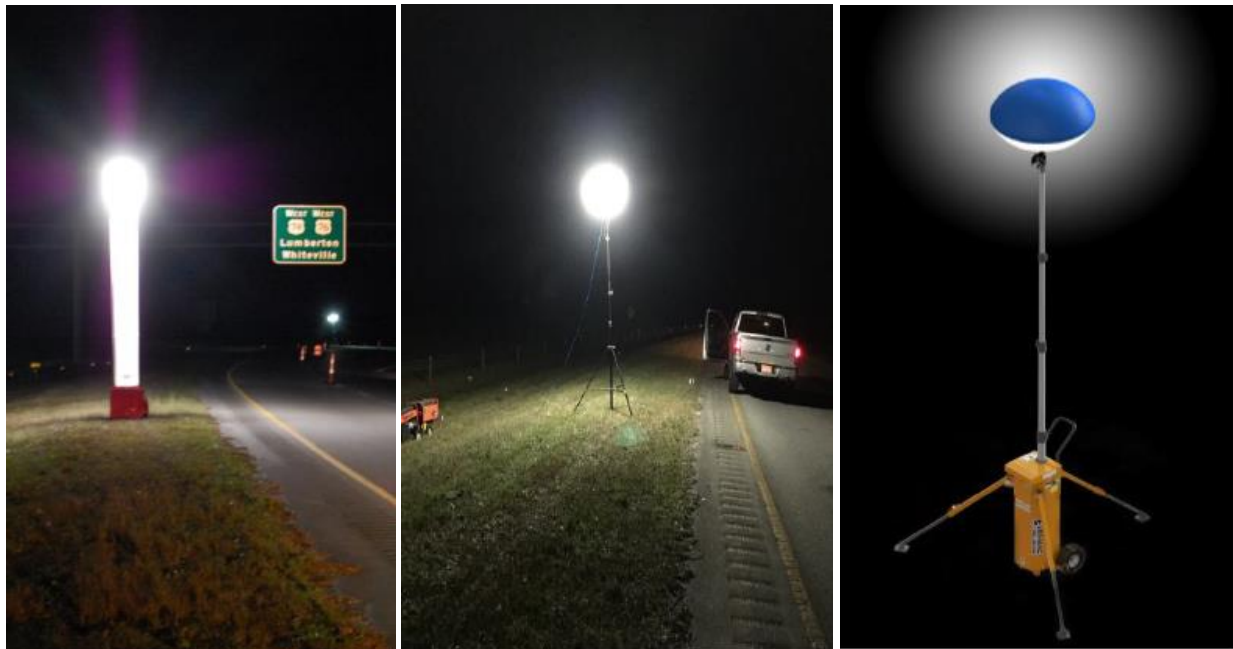
Figure 25. Various Presence Lighting Fixtures
