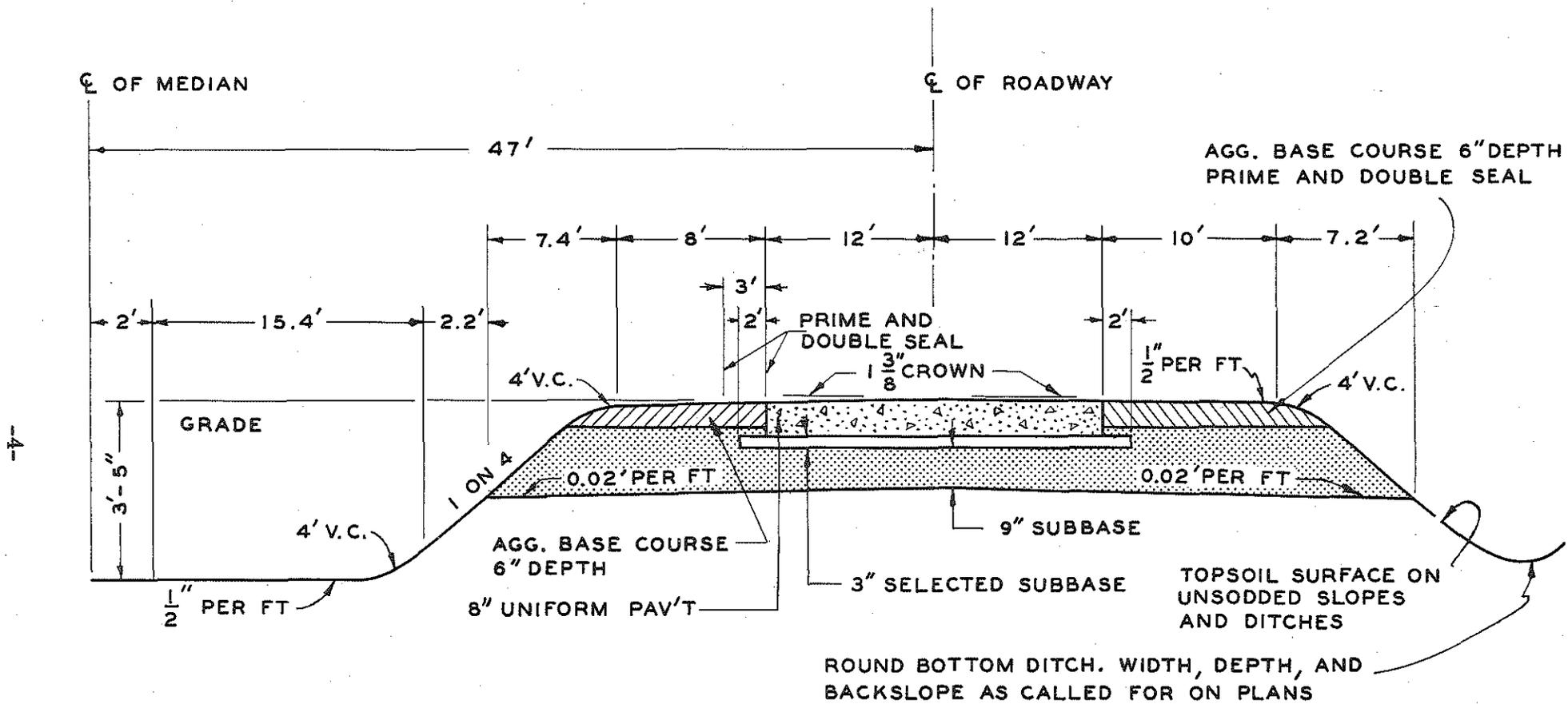
Figure 2. Typical road cross-section.
