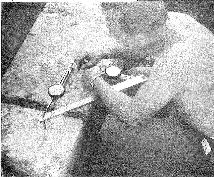
▼ Figure 44. Measuring sectional slab displacement with vernier calipers and invar tape.
