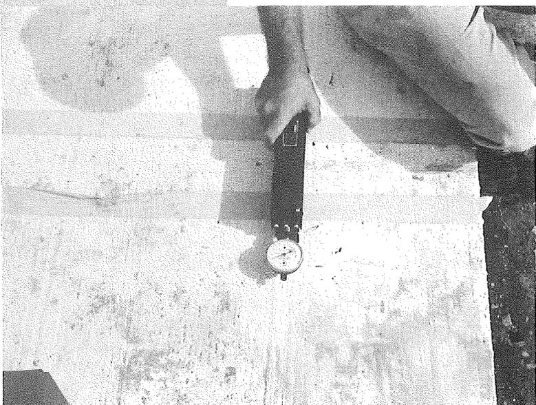
▶ Figure 47. Measuring crack opening with Whittemore strain gage.
