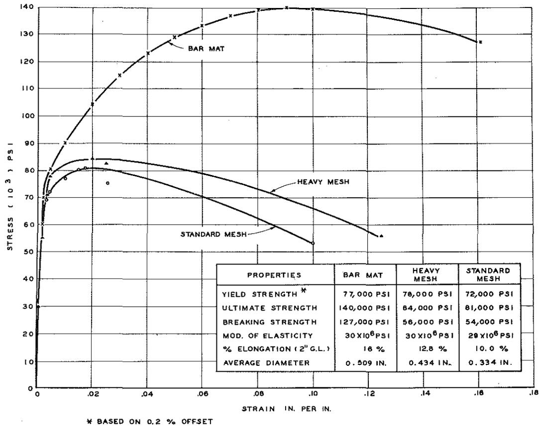
Figure 50. Steel reinforcement properties.
