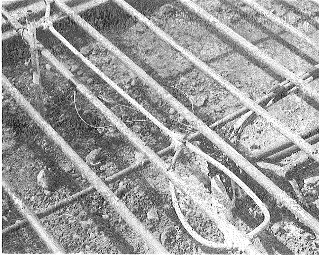
Figure 34. Instrumented wire mesh reinforcement with corrugated crack former and thermocouples.
