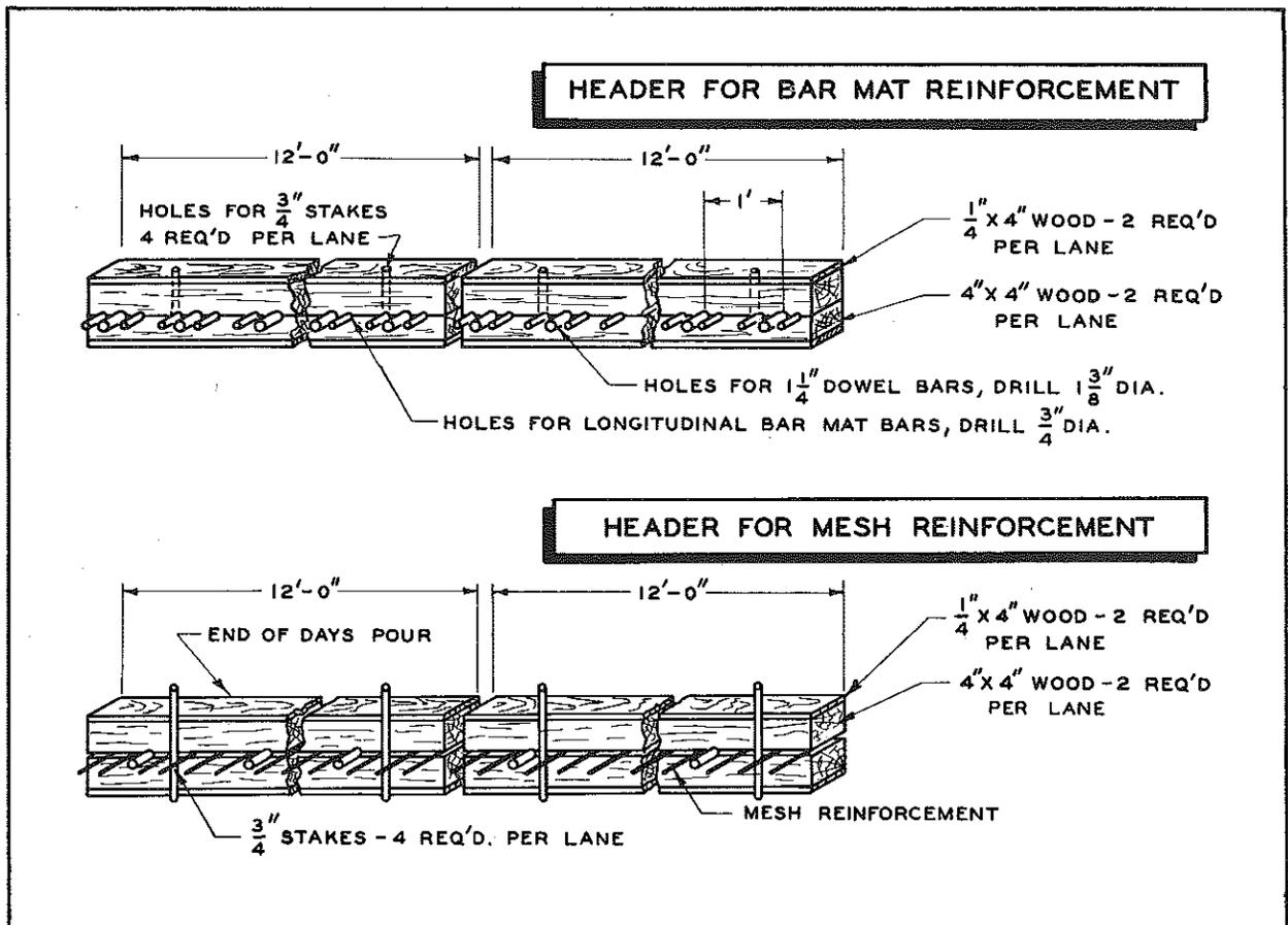
Figure 18. Details of construction joint headers.
