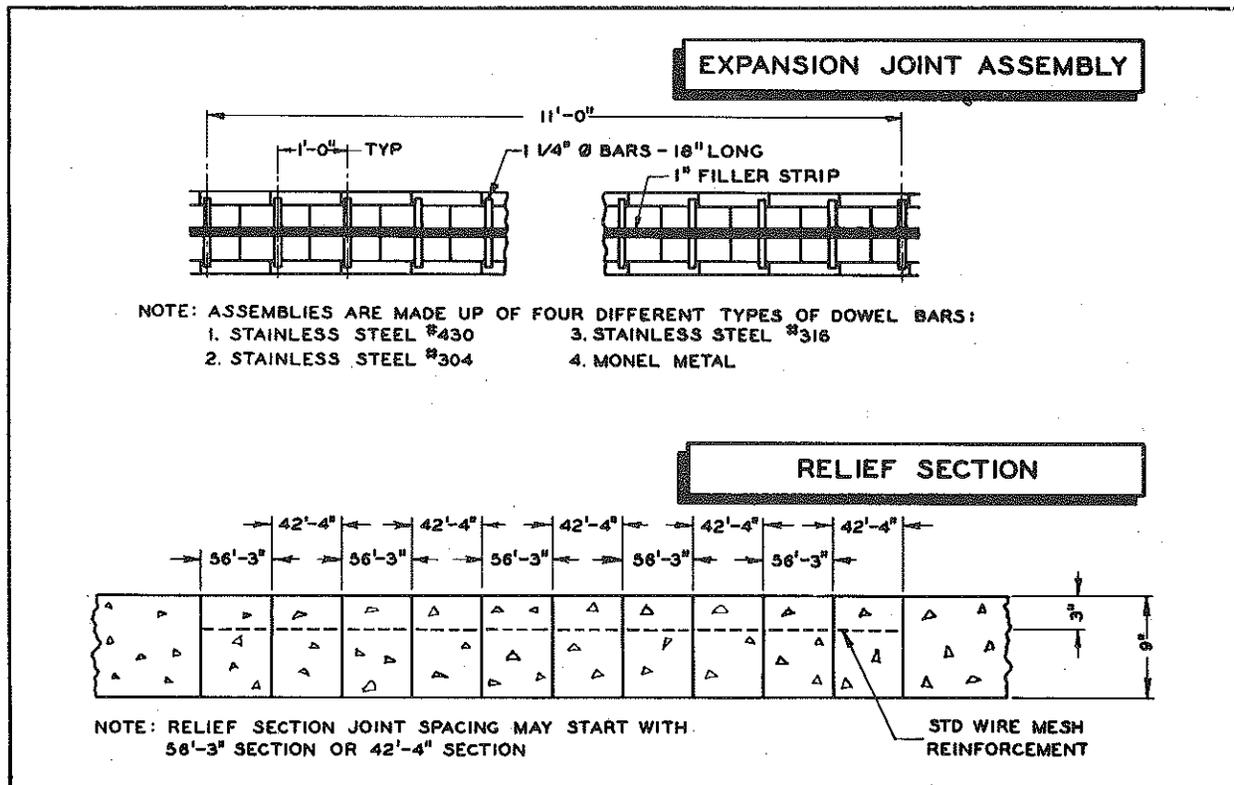
Figure 4. Typical expansion joint assembly and relief section.
