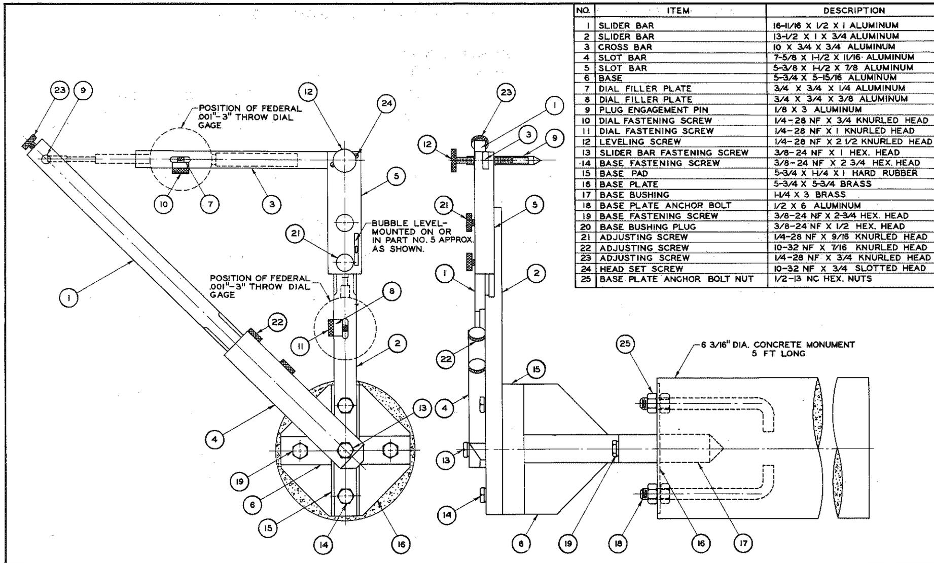
Figure 25. Assembly drawing of pavement displacemeter.
