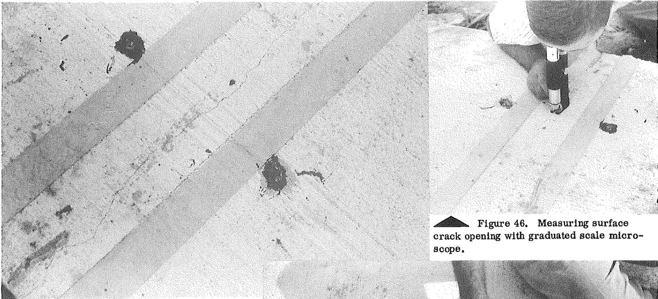
▲ Figure 45. Plugs set in epoxy resin for crack opening measurements.
