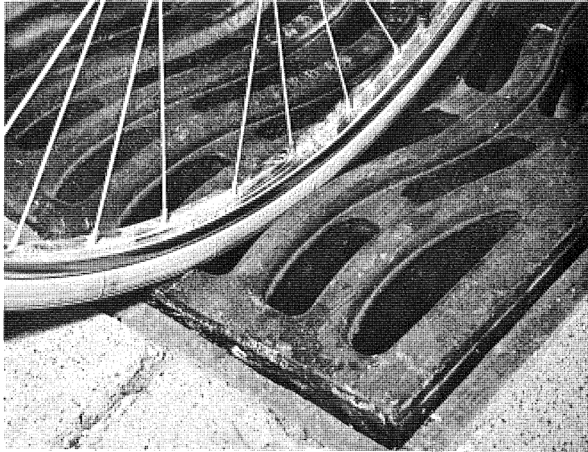
Figure 1. Modified Sinusoidal Type A Grating showing that the narrow bicycle tire rides on the cross-bracing and does not penetrate the grating opening.
