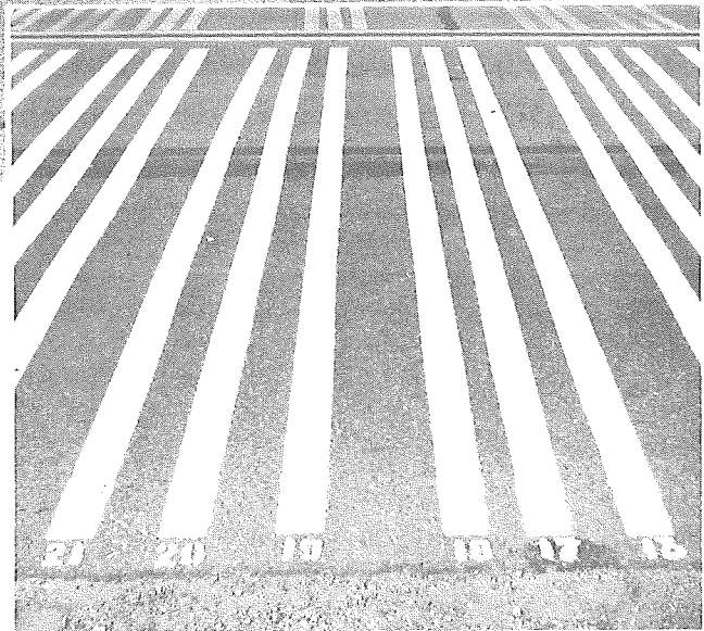
Figure 2. Initial appearance of stripes in Test Area 4 (bituminous) on M 43 near Okemos (above), with yellows in foreground and whites in background. Close view of some white stripes is shown at right.
