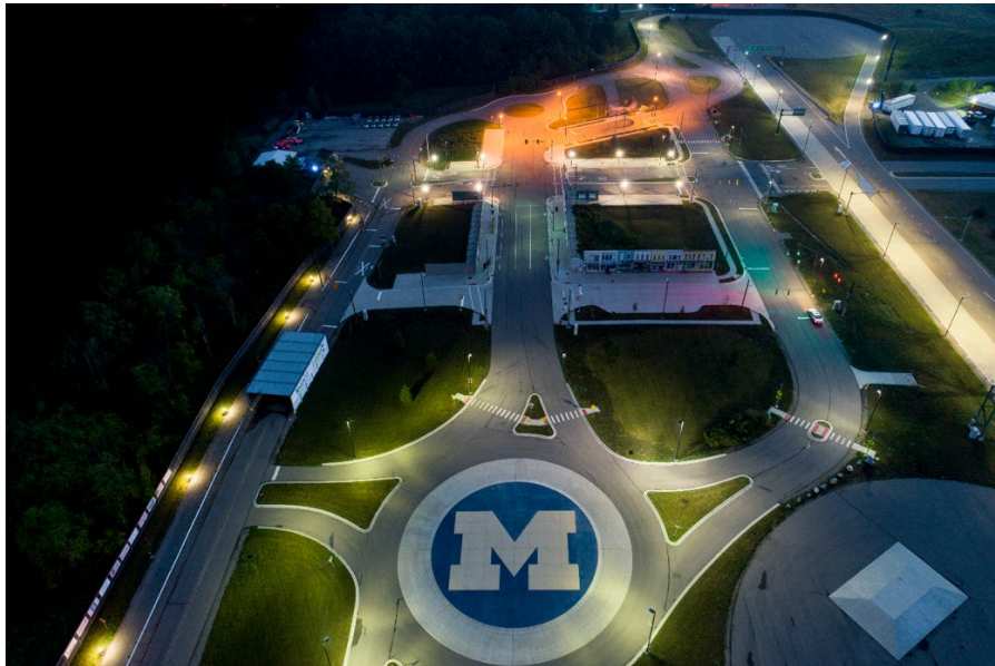
Figure 6: Aerial photo of the Mcity Test Facility as originally constructed, at dusk when various types and color temperatures of roadway lighting are evident.
