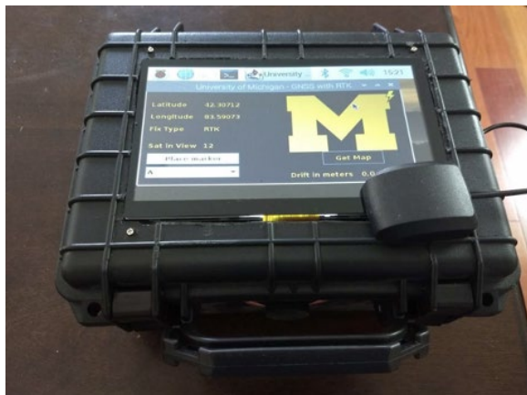
Figure 32: Mcity's RTK unit for vehicles.
