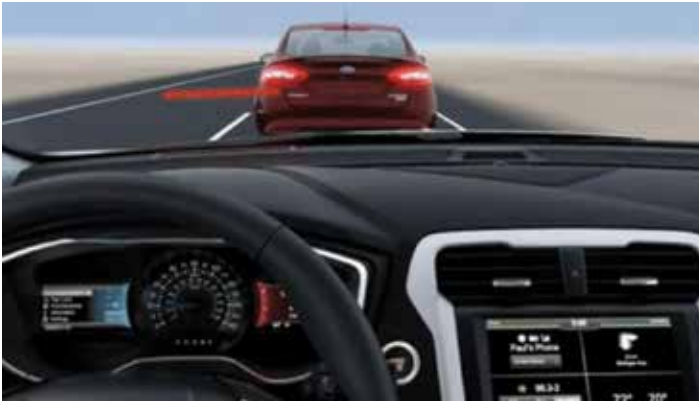
Figure 3-3 Collision Detection Braking of Ford (Ford 2016)
