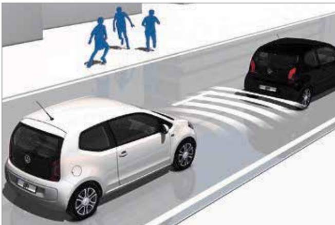
Figure 3-1 Autonomous Emergency Braking (Volkswagen 2011)
