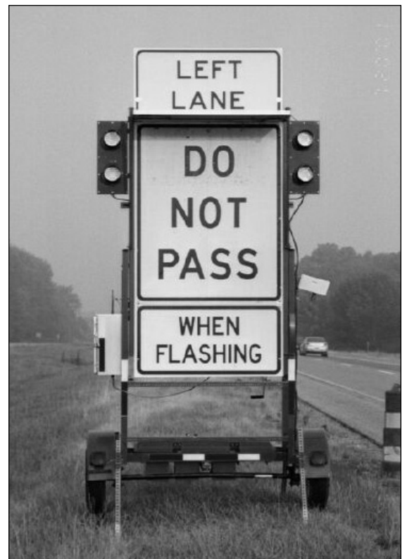
Figure 1. The DO NOT PASS WHEN FLASHING Sign is an Important Part of the DLMS.
