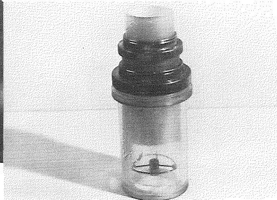
FIGURE 7. BETA GAGE SHOWING SOURCE HOLDER, PLASTIC CYLINDERS AND BRASS FRICTION RINGS COMPRISING INTERIOR - ASSEMBLED.
