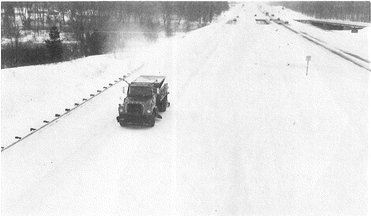
CMA application on test section is the dark band behind the truck near the centerline.
