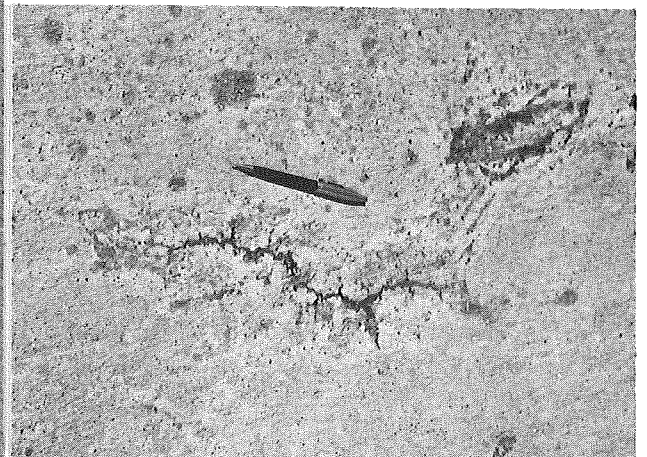
Figure 4. General view (left) of shrinkage cracks in middle portion of silicone Pour A, with close view of typical crack (below).
