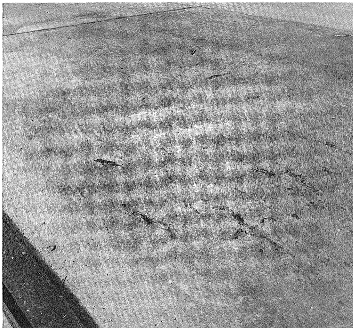
Figure 4. General view (left) of shrinkage cracks in middle portion of silicone Pour A, with close view of typical crack (below).
