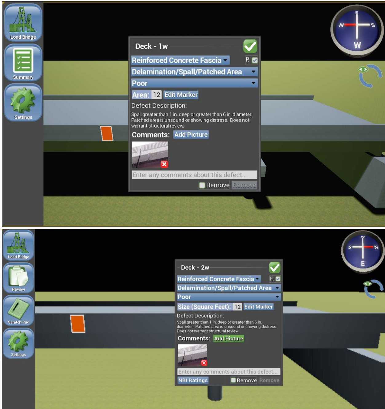
Figure 6-5: Defect pop-up menu. Title and element shortlist are context-sensitive according to the bridge location touched.
