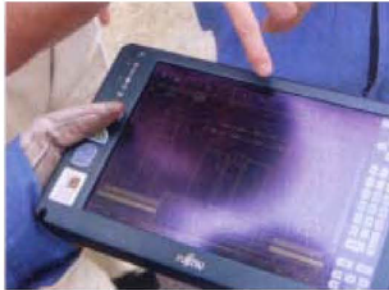
Figure 6. An example of a handheld tablet device that allows inspectors to make on-site updates to bridge inspection records when using Advitam ScanPrint.
