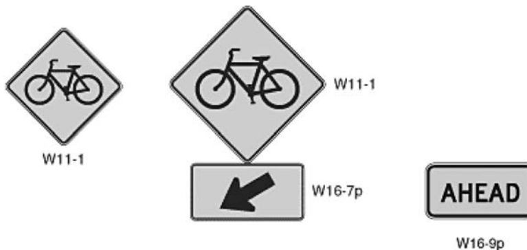
EXHIBIT V-10 Bicycle Warning Signs (USDOT, 2003)
