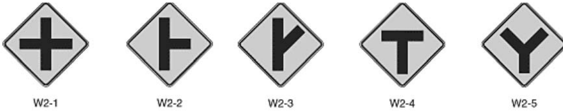
EXHIBIT V-8 Intersection Warning Signs (USDOT, 2003)
