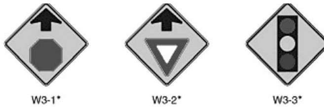
EXHIBIT V-9 Advance Traffic Control Signs (USDOT, 2003)
