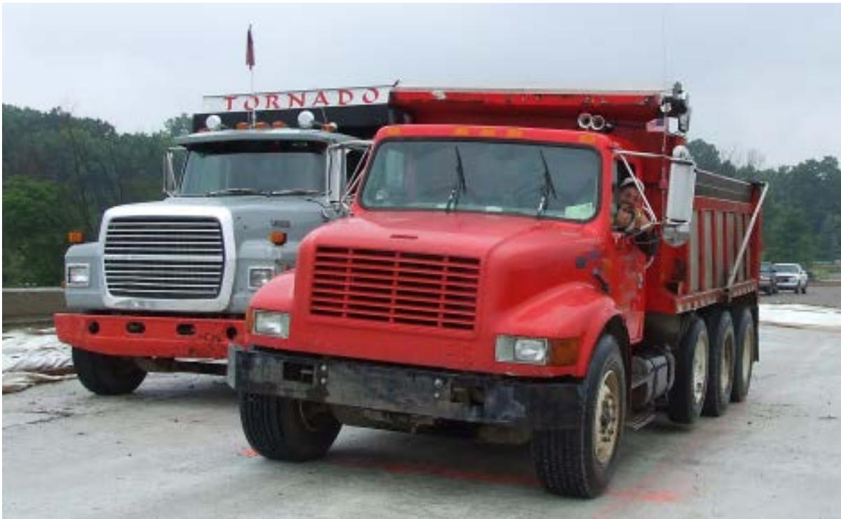
Figure 3.21 3-axle trucks used to load Woodruff Bridge
