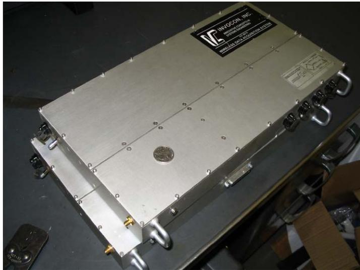
Figure 3.5 Radio-based Invocon strain data acquisition system
