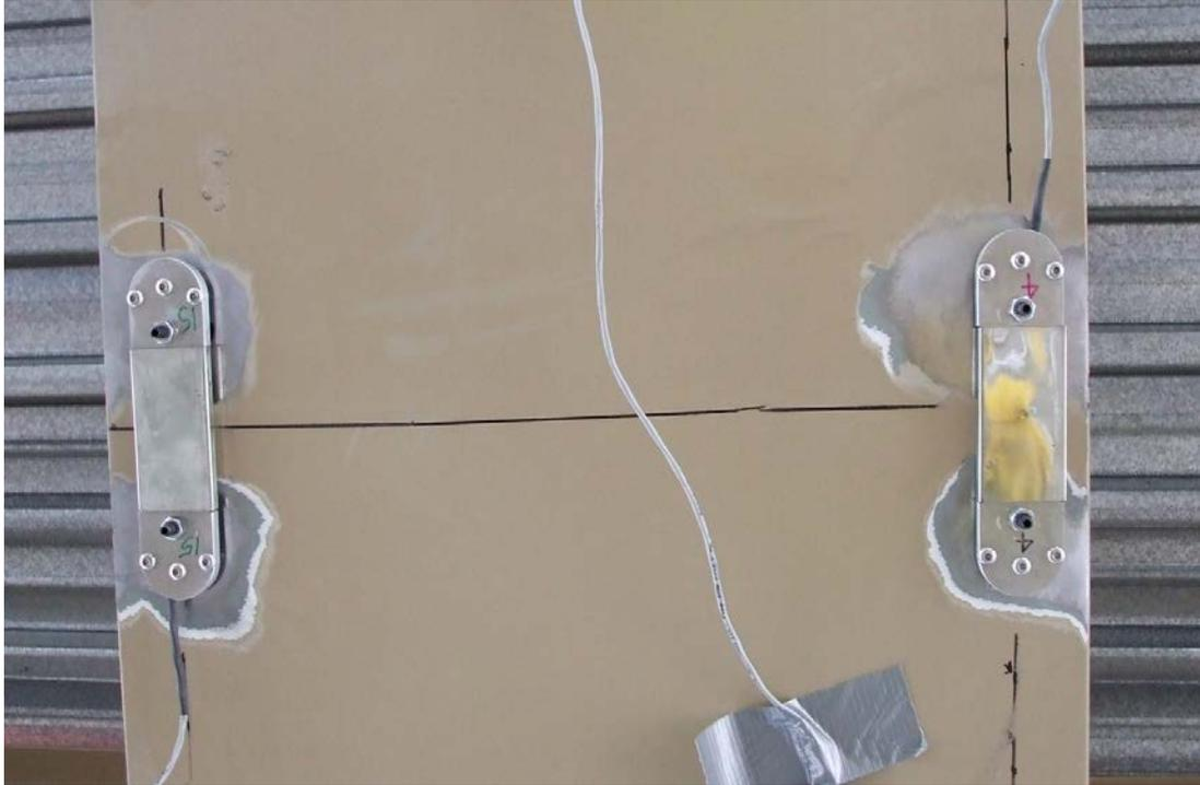
Figure 3.8 Strain transducer arrangement on bottom flange at Locations S1 and S2
