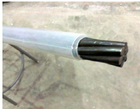
Traditional soft sheathing on the ends of prestressing strands (left) was not producing the desired debonding effect in bridge beams. The use of rigid tubing (right) as an alternative made the difference.
