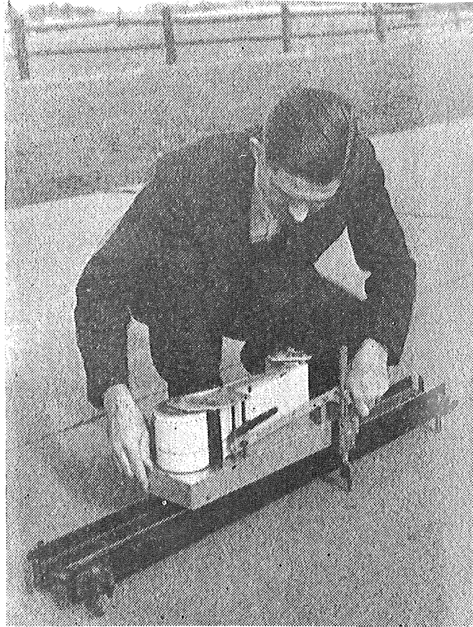
Figure 3. Small Profilometer with Fixed Datum
