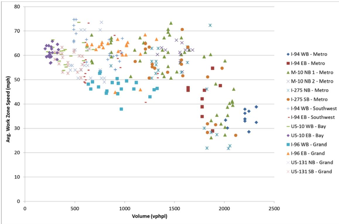
**Figure 18. Combined Work Zone Speed-Flow Curve**
