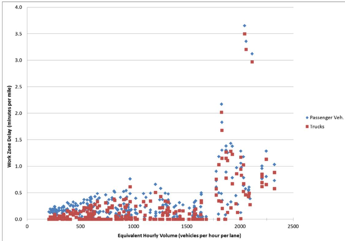
**Figure 22. Normalized Work Zone Delay vs. Equivalent Hourly Volume per Lane**
