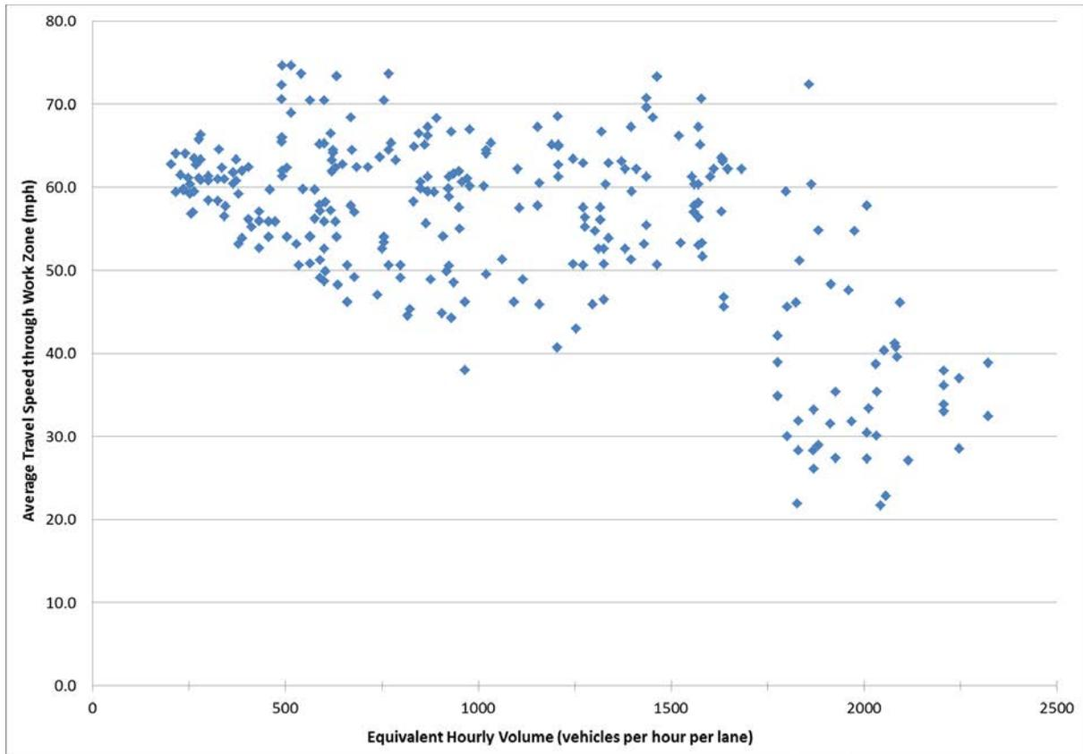
**Figure 17. Average Work Zone Travel Speed vs. Equivalent Hourly Volume per Lane**
