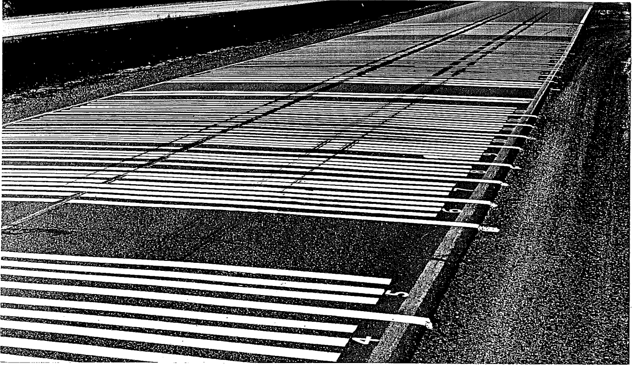
Figure 1. Test stripes on WB M 78 (Bituminous) with whites in foreground and yellows in background. Stripes were laid immediately West of last year's. Photo taken 5/23/72, 4 days after application, shows skid-marks of vandal's vehicle. Later, the other area was similarly vandalized, as were previous tests in the St. Johns area.
