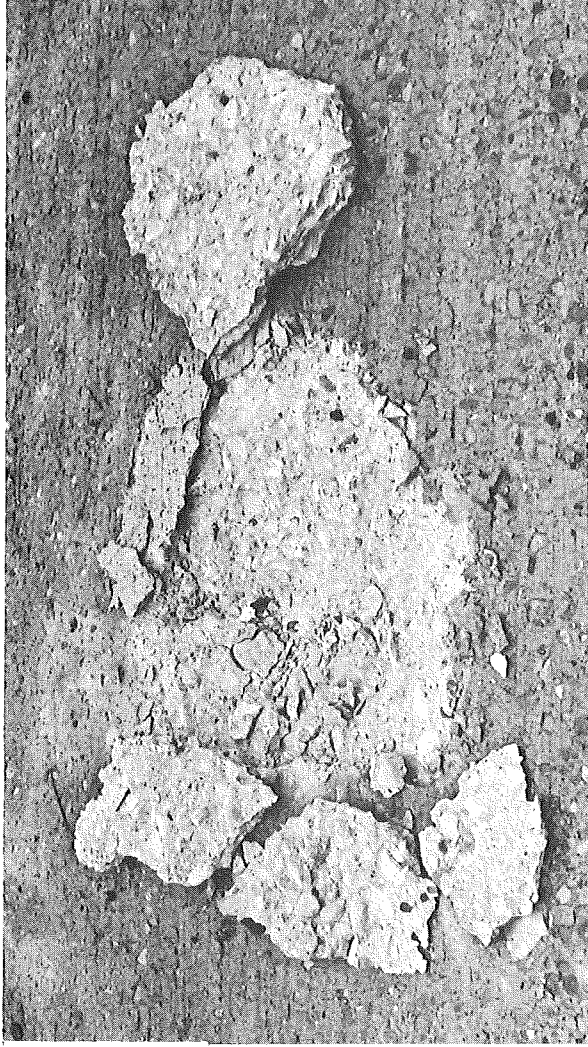
Figure 2. Concrete after extraction of Kwik-Bolt, where expansion sleeves remained in the hole and little concrete damage occurred. ▽
