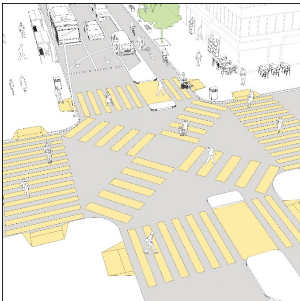
Traffic signal with exclusive pedestrian phasing or pedestrian scramble (Global Designing Cities Initiative n.d.)
