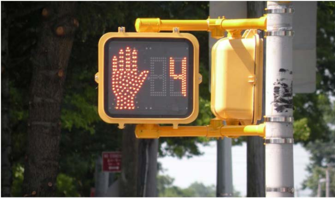
Traffic signal with pedestrian countdown signal (Chicago Metropolitan Agency for Planning n.d.)
