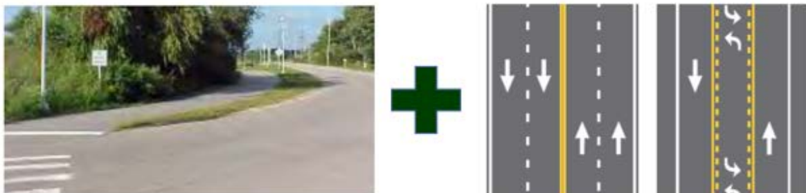
Sidepath (Michigan Department of Transportation 2014a) + Lane reduction (Michigan Department of Transportation 2019)
