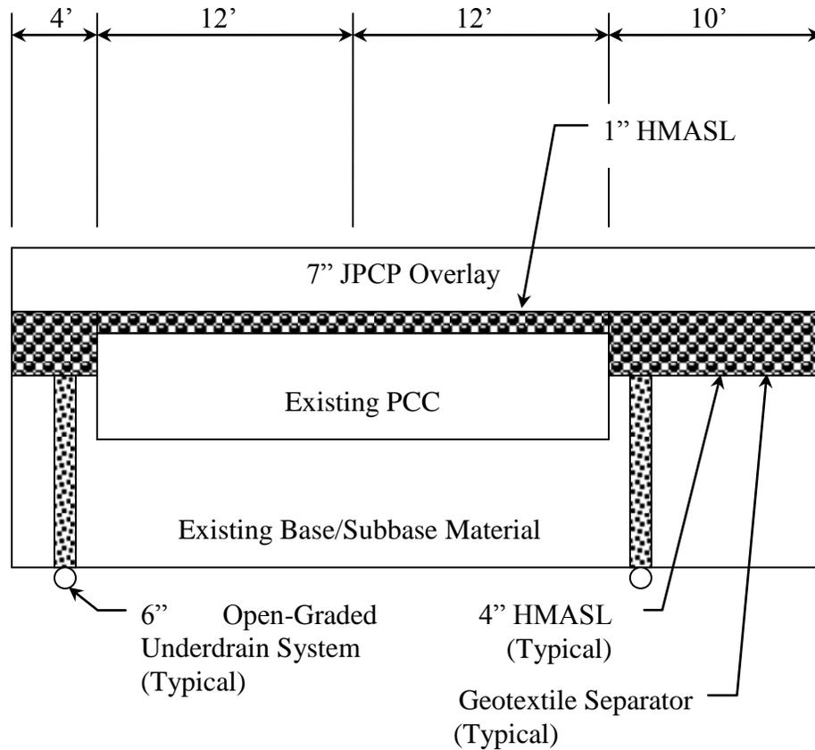
Figure 5.1 New Overlay Drainage System: Thickened Shoulder Design with Open-Graded Underdrains (depending on soil conditions).
