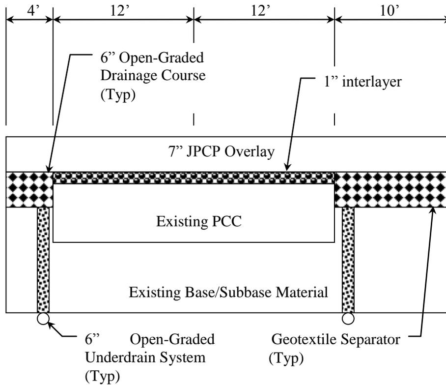
Figure 5.2 New Overlay Drainage System: OGDC Shoulder Design
