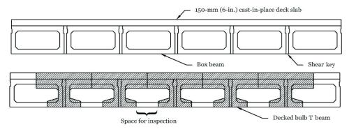
Researchers proposed modifying traditional side-by-side, box-beam bridge superstructures (top) with decked bulb T beams (bottom).
