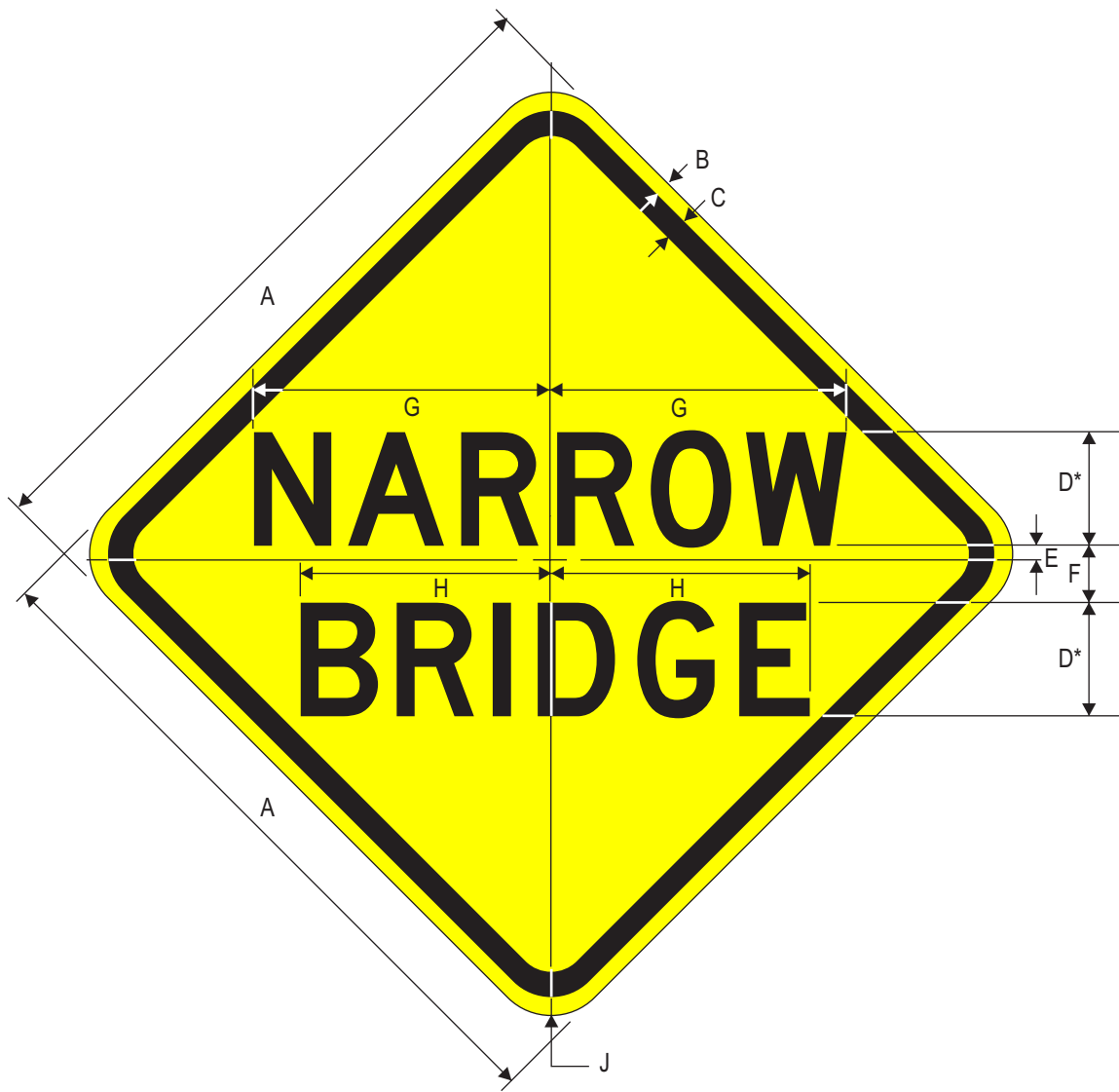
W5-2 NARROW BRIDGE
