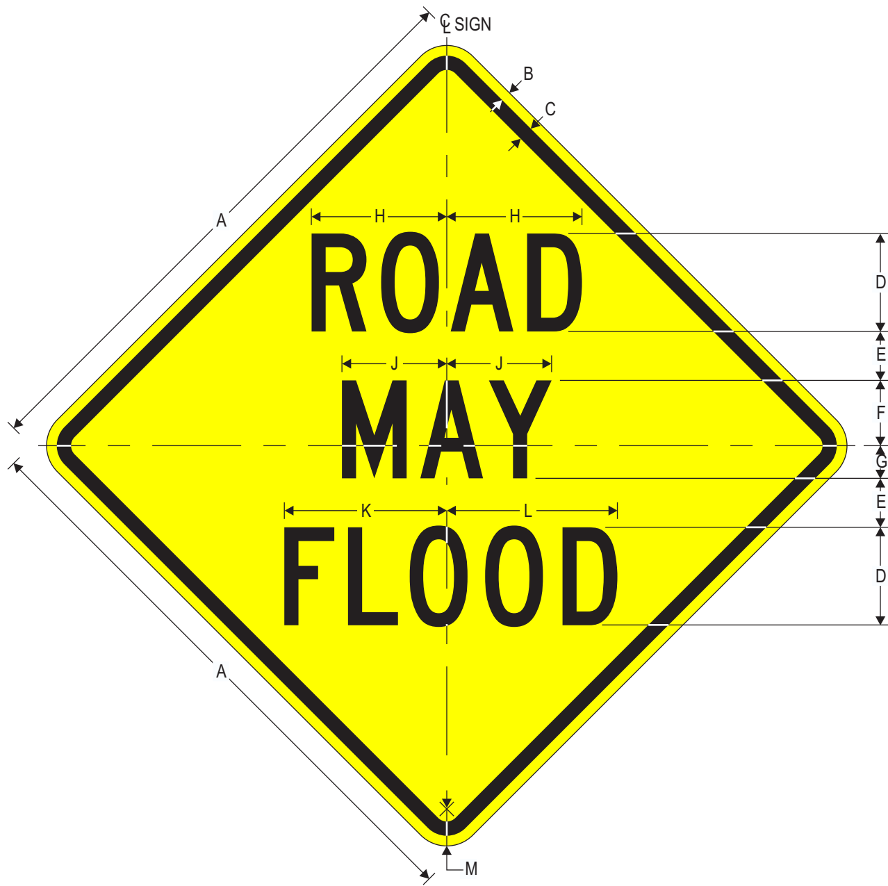
W8-18 ROAD MAY FLOOD
