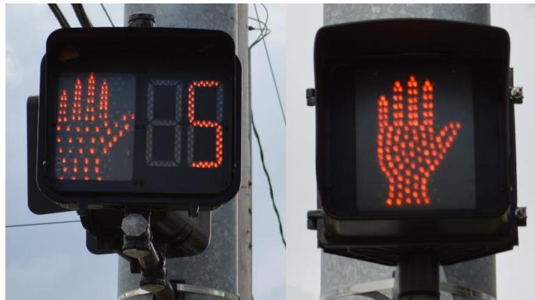
**Figure 2.2 Pedestrian countdown signal (left) vs. standard pedestrian signal (right)**
