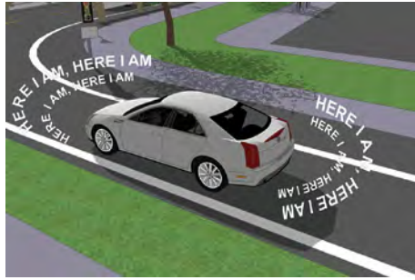
Wireless connectivity allows cars to tell other vehicles where they are located at all times. (Courtesy of U.S. DOT.)
